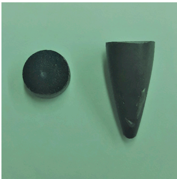
Fig. 1. Grown \text{AgIn}_5\text{S}_8 single crystals.
